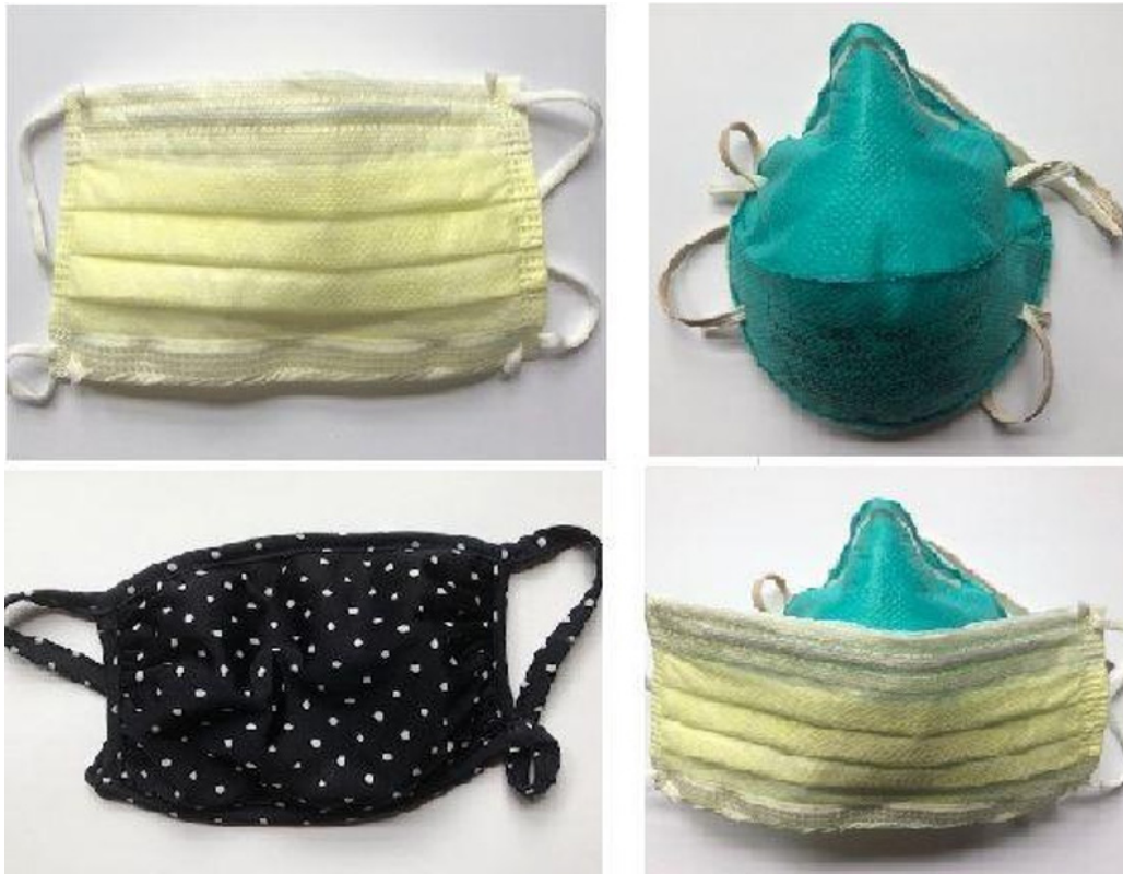
Figure 8: Picture of face masks used. Surgical mask (top left), N95 mask (top right), Cloth mask (bottom left), Surgical mask on top of N95 mask (bottom right).
