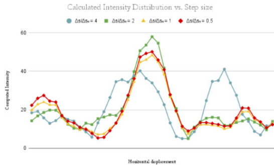
Figure 5: Calculated intensity distribution vs. Step size. Figure graphically depicts the convergence of predicted intensity as grid spacing is decreased.
